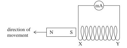
A current is produced in the coil, which creates a magnetic field around the coil.
