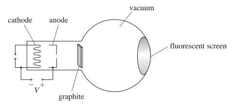
A potential difference V was applied between the cathode and the anode to produce the beam of electrons.
