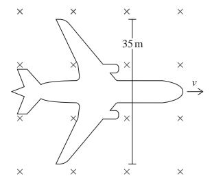
An e.m.f. of  $0.40\,\mathrm{V}$  is induced across the wing tips. The pilot states that the aeroplane is flying with a speed of  $250\,\mathrm{m\,s^{-1}}$ .
