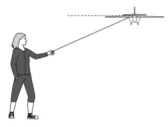
The aeroplane moves in a horizontal circle of radius  $28.5 \,\mathrm{m}$  at a speed of  $22.5 \,\mathrm{m\,s}^{-1}$ . A lift force acts vertically upwards on the aeroplane. The lift force is equal to twice the weight of the aeroplane.
