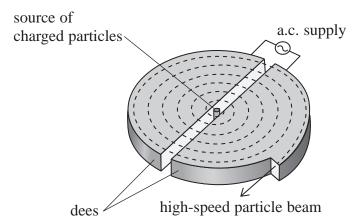
(i) Explain how the cyclotron produces a beam of high energy particles.
